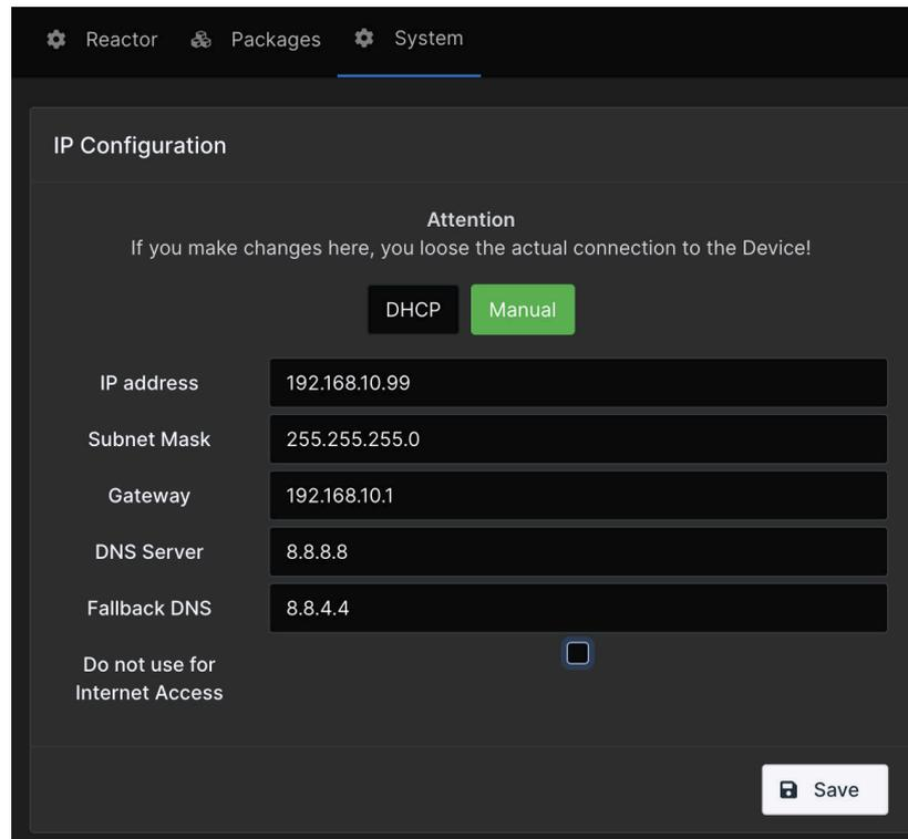
The screenshot shows the 'System' menu with 'IP Configuration' selected. At the top, there are navigation options: 'Reactor', 'Packages', and 'System'. Below the title, an 'Attention' warning states: 'If you make changes here, you loose the actual connection to the Device!'. There are two buttons: 'DHCP' (disabled) and 'Manual' (active). The configuration fields are as follows:
